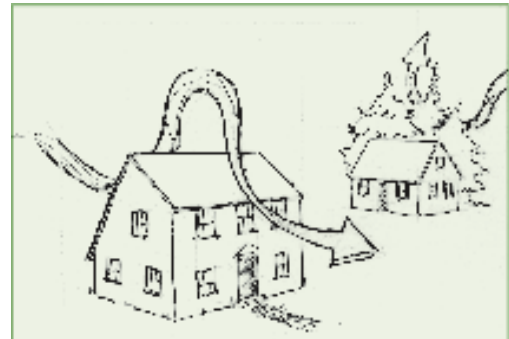
Historic building types and style, like the classic saltboxes of New England, were designed and oriented to maximize solar gain and reduce wind chill. Printed in "Energy Efficiency, Renewable Energy and Historic Preservation: A Guide for Historic District Commissions."
